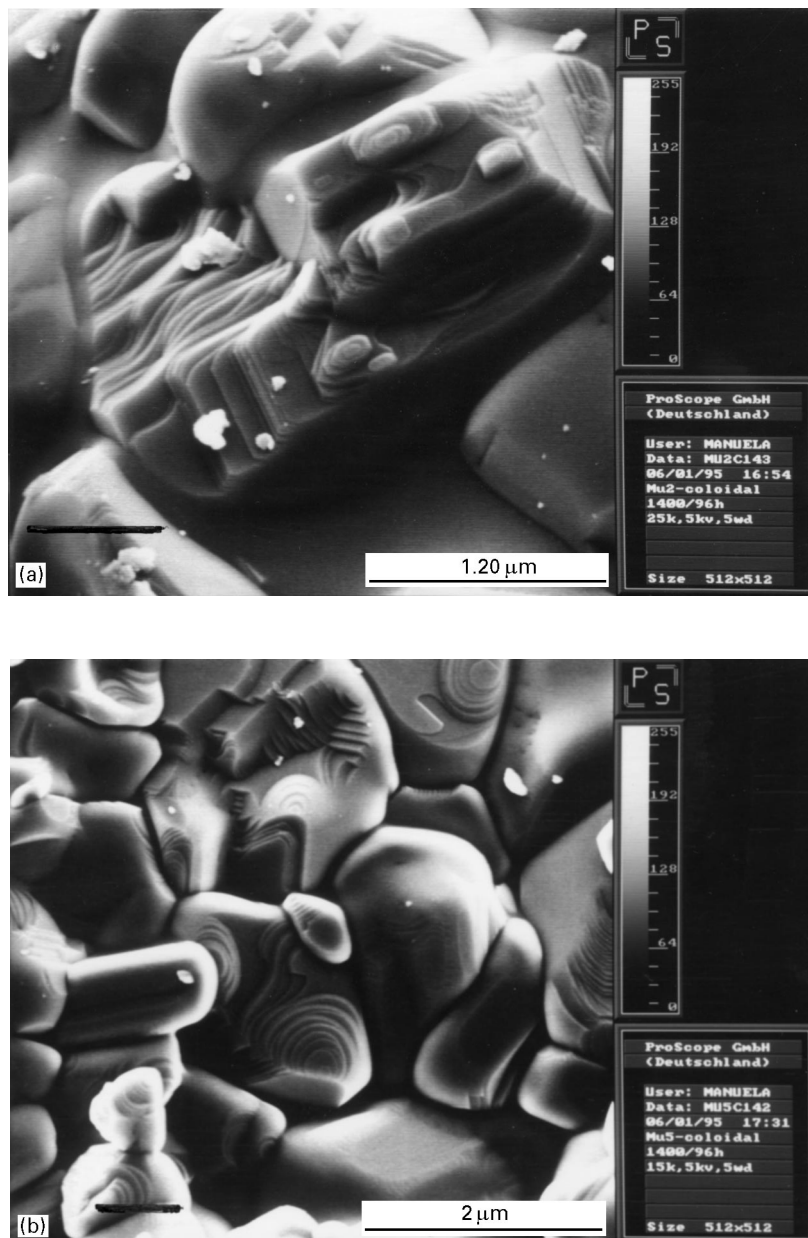
Figure 7 Scanning electron micrographs of colloidal gels heat treated at 1400 °C/96 h: (a) CGB, (b) CGD.
